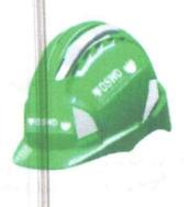
Safety Helmet specification: At least 85% polyamide, UPF-50 or High-density HDPE or ABS shell. With airhole, reflectorized sticker, quick drying with perforations around temples, with adjustable/removable band and soft PVC chin Strip, water, stain and impact proof.
