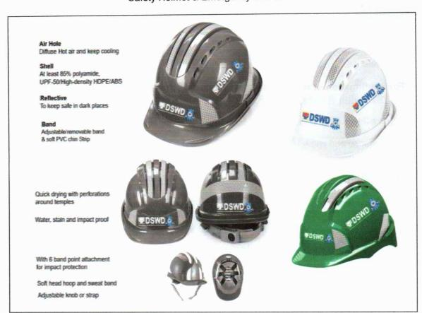
**Safety Helmet specification**: At least 85% polyamide, UPF-50 or High-density HDPE or ABS shell. With airhole, reflectorized sticker, quick drying with perforations around temples, with adjustable/removable band and soft PVC chin Strip, water, stain and impact proof.
